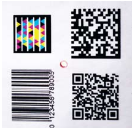
The Bokode device, at center, is much smaller than other types of barcodes, yet can contain far more information. Photo courtesy Media Lab Camera Culture group
